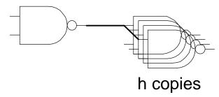
□ Estimate rising and falling propagation delays of a 2-input NAND driving h identical gates.
