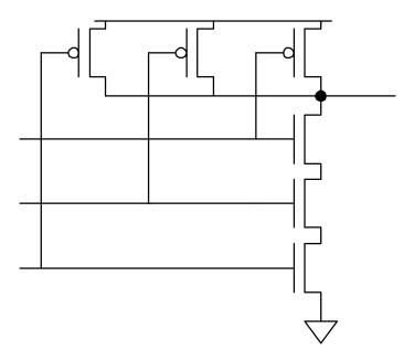
□ Sketch a 3-input NAND with transistor widths chosen to achieve effective rise and fall resistances equal to a unit inverter (R).
