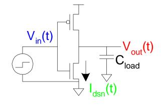
$$I_{dsn}(t) = \begin{cases} 0 & t \leq t_0 \\ \frac{b}{2} \left( V_{DD} - V \right)^2 & V_{out} > V_{DD} - V_t \\ b \left( V_{DD} - V_t - \frac{V_{out}(t)}{2} \right) V_{out}(t) & V_{out} < V_{DD} - V_t \end{cases}$$
